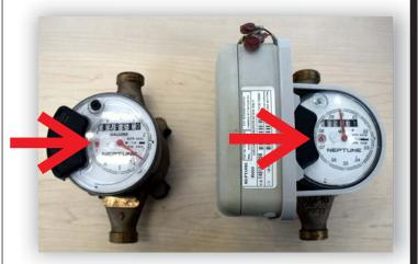
If orange triangle is spinning, water is flowing
