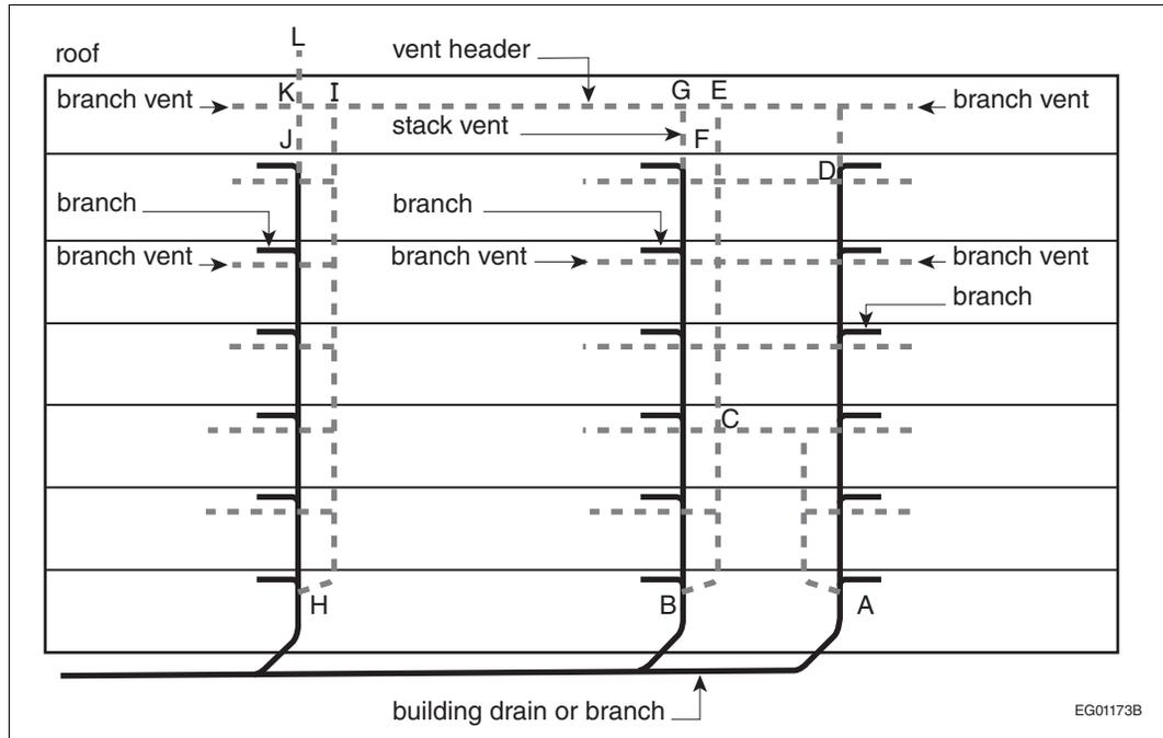
**Figure A-2.5.8.3. and 2.5.8.4.-B****Lengths to be considered when sizing stack vent, vent stack and vent header pipes****Notes to Figure A-2.5.8.3. and 2.5.8.4.-B:**
