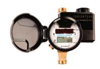
Shine a flashlight over the solar panel on the register to activate the LCD display. The display will switch between the flow rate and total consumption every six seconds.
