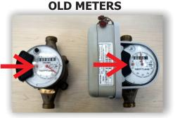
If orange triangle is spinning, water is flowing
